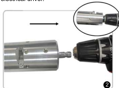
Attach the trimming tool to power drill.
