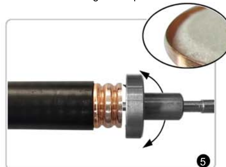
Use BXD07-6 to reshape the outer corrugation. Make sure to put the two shaping teeth inside the corrugation and then rotate until the outer corrugation is round enough with no dent or deformation and create visible clearance between outer corrugation and inner insulator.
